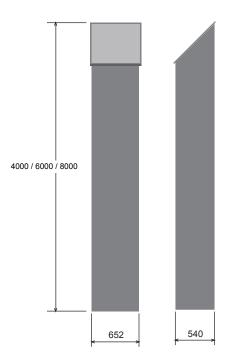
Possibility to customise with logos and texts / Use of corten steel, no treatments or maintenance needed / LED backlighting / Vandalproof. Dawn and dusk dimming.
